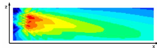
Figure 13 **Vertical sound intensity distribution of a line array with adjusted near-field for different distances to the listening area**
