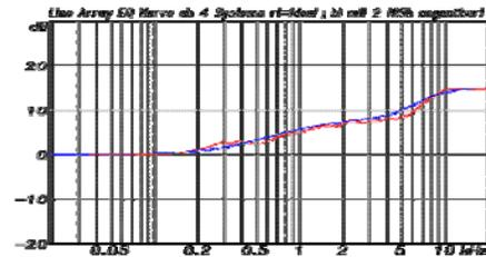
Figure 17 Typical filter to compensate for the coupling in the bass range
