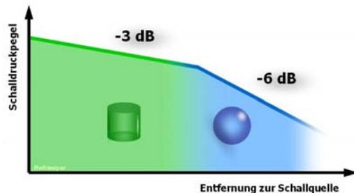
Figure 7 Sound intensity gradient in near-field and far-field
