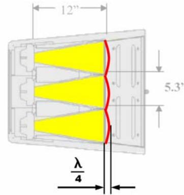
Figure 8 Curving of the wave-fronts
