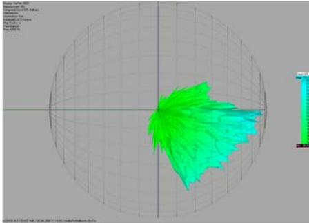
Figure 14 **Vertical radiation behaviour of a long line-array**
