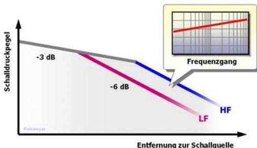
Figure 10 Transition from near-field to far-field for a straight linear transducer at different frequencies
